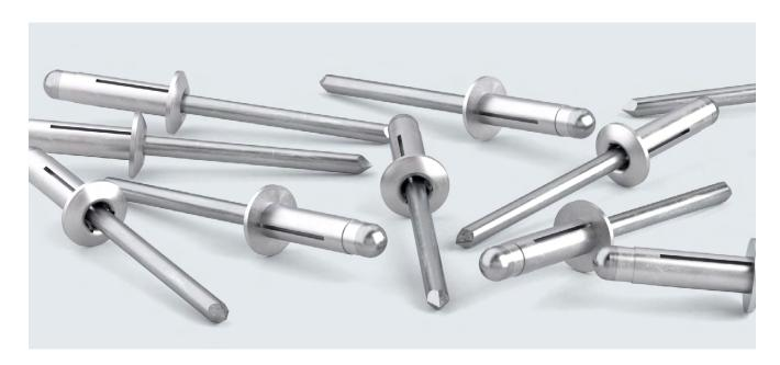
TIFAS® Star blind rivets form three folding legs on the blind side on installation. These large-shaped folding legs evenly and sparingly distribute the resulting clamp force across the riveted material.
