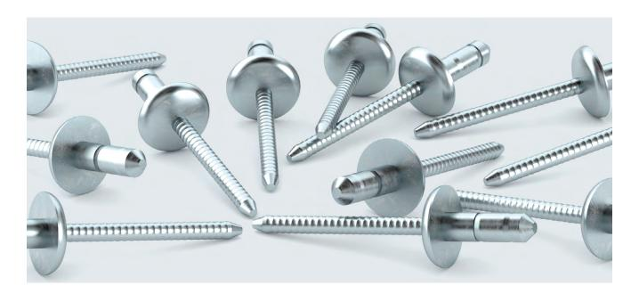
The combination of a consistently large blind-side footprint, vibration resistance and a partially load-bearing as well as securely retained mandrel make the TIFAS\* Grip blind rivet the ideal choice for thin components that need to withstand high loads. The application of bearing pressure compensates for drilled hole tolerances.
