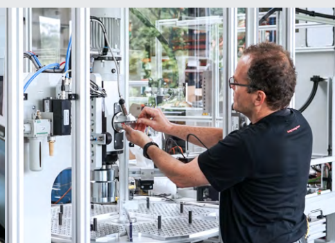
FMW riveting machine assembly in a CNC indexing table machine
